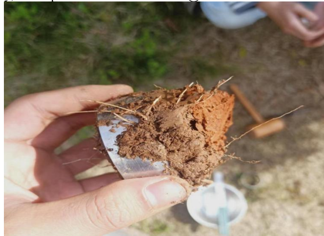
Figure 8. The Natural Root System Collected By The Ring Knife
