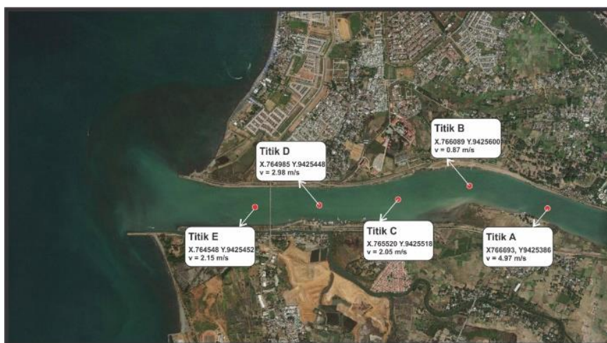
Figure 4. Location of Flow Velocity Measurement
